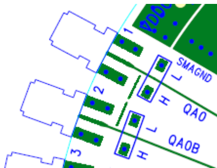
Figure 4. LVPECL Output Configuration
