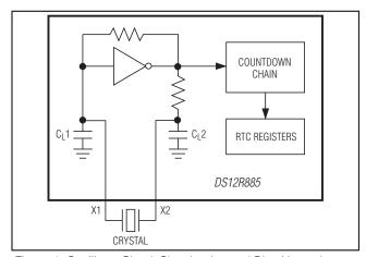
Figure 1. Oscillator Circuit Showing Internal Bias Network
