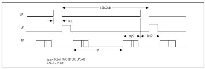
Figure 3. UIP and Periodic Interrupt Timing
