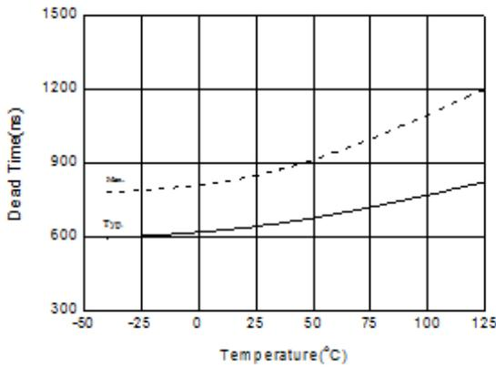
Figure 57. Deadtime vs. Temperature ( $V_{CC}=V_{BS}=15\text{ V}$ ,  $V_{DT}=1.2\text{ V}$ )
