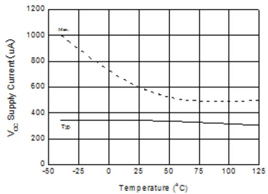
Figure 44.  $V_{CC}$  Supply Current vs. Temperature ( $V_{CC}=15\text{ V}$ )
