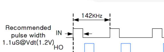
Figure 7. Recommendation of Pulse width Output Waveform
