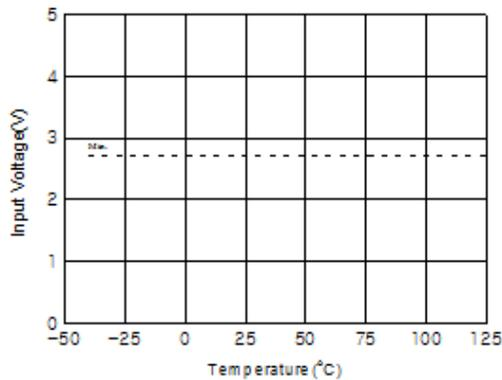
Figure 31. Logic Low Input Voltage vs. Temperature
