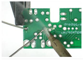
Now solder both wires to the PCB.
