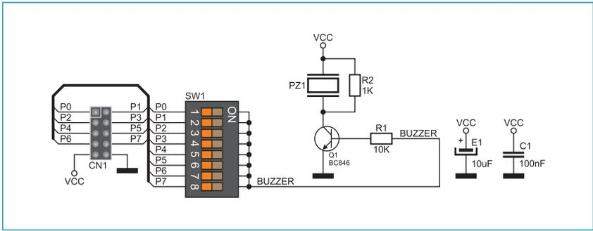
Figure 2: EasyBuzz additional board connection schematic
