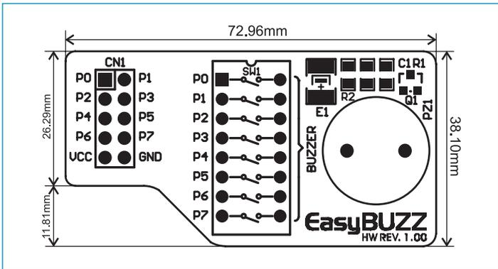
Figure 3: Dimensions of the EasyBuzz additional board
