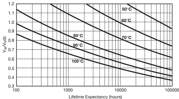
V<sub>w</sub> = Permanent working or operating DC voltage.
