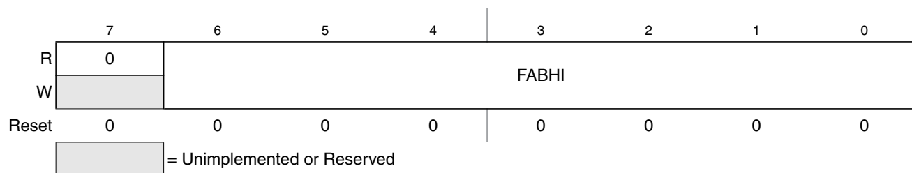
Figure 19-16. Flash Address High Register (FADDRHI)
