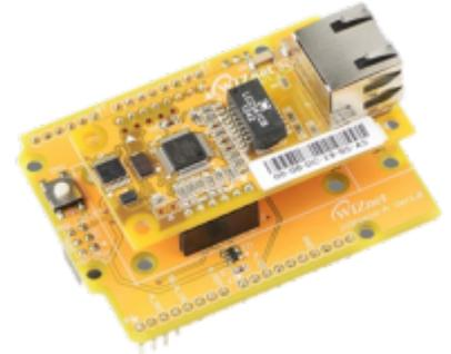
It is based on the [WIZ550io network module](#) which uses [WIZnet W5500 ethernet chip \(W5500 Datasheet\)](#). The WIZnet W5500 provides a network (TCP/IP) stack capable of both TCP and UDP. It supports up to eight simultaneous socket connections. And, when Powered on and nRESET triggered, WIZ550io initializes itself with embedded real MAC and default IP address and can be pinged from user's computer.
