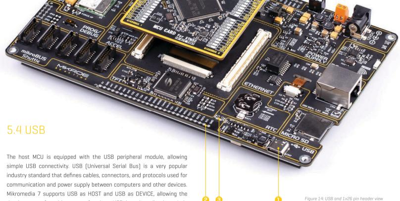
development of a wide range of various USB-based applications. It is equipped with the USB-C connector [1], which offers many advantages, compared to earlier types of USB connectors (symmetrical design, higher current rating, compact size, etc).
