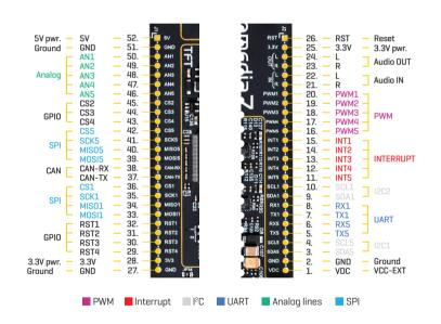
Figure 15: 1x26 pin header view
