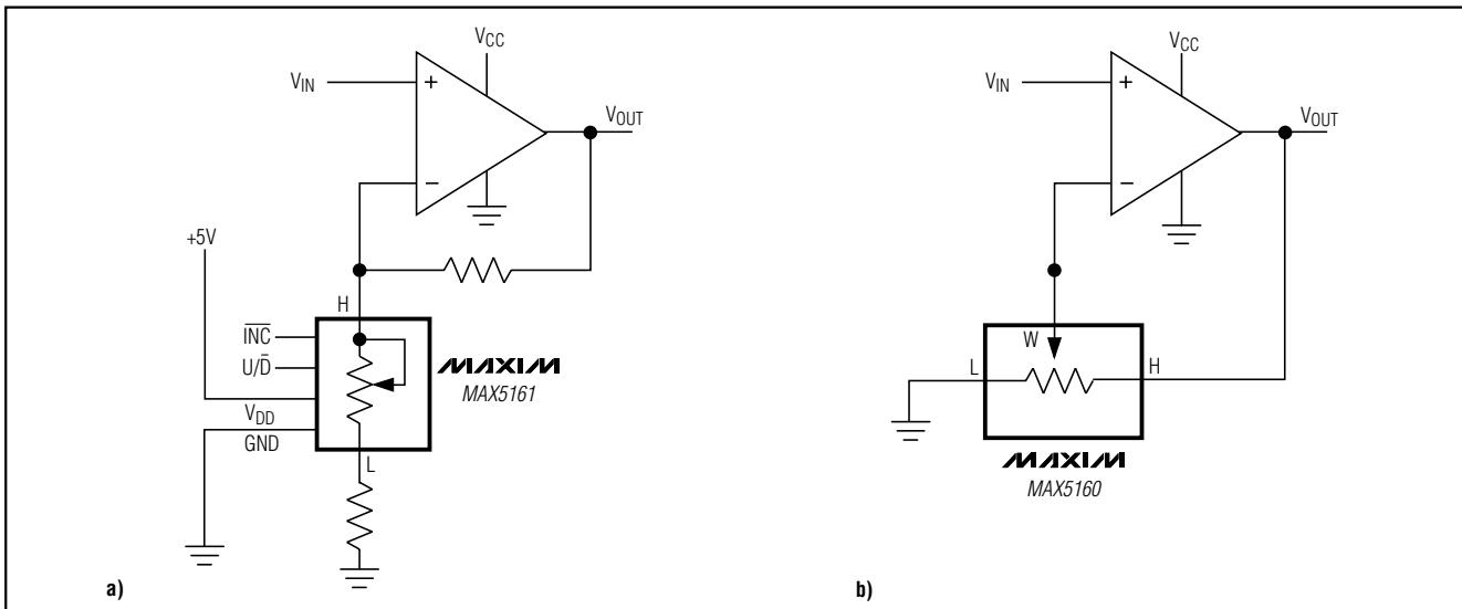
Figure 5. Adjustable Gain Circuit: a) MAX5161; b) MAX5160
