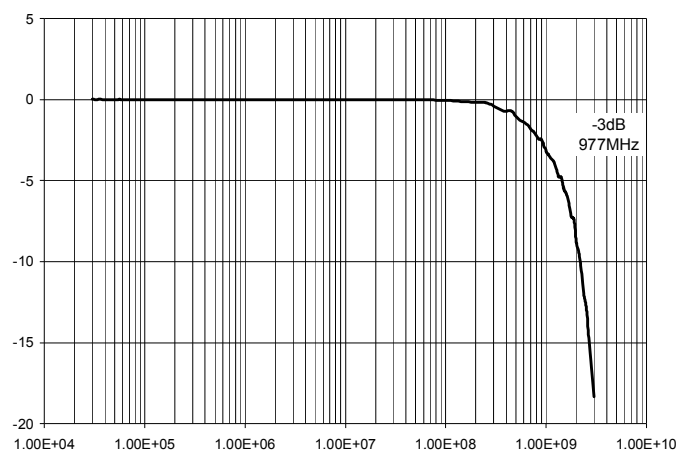
Typical Insertion Loss (S21) 30KHz to 3GHz
