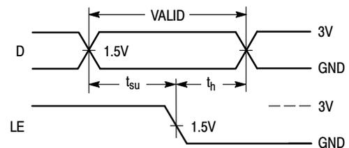
Figure 6. Switching Waveform
