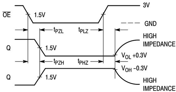
Figure 5. Switching Waveform
