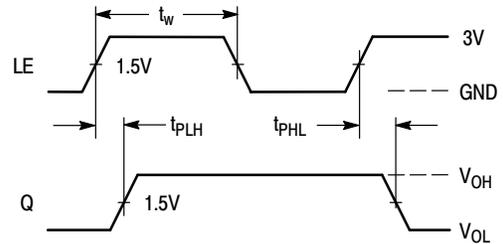
Figure 4. Switching Waveform
