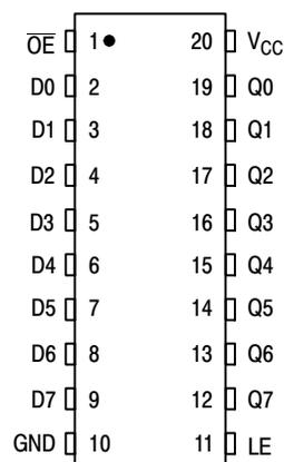
Figure 2. Pin Assignment
