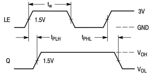
Figure 4. Switching Waveform
