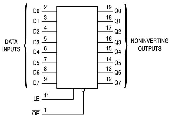
Figure 1. Logic Diagram
