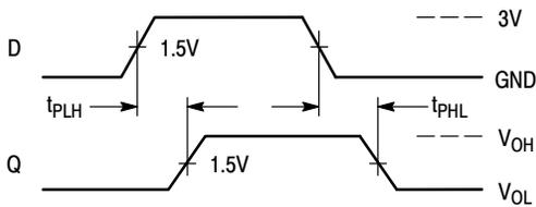
Figure 3. Switching Waveform
