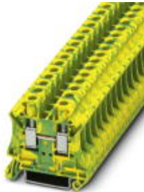
Feed-through terminal block, Connection method: Screw connection, Cross section: 0.2 mm 2 - 10 mm 2 , AWG 24 - 8, Width: 8.2 mm, Color: green-yellow, Mounting type: NS 35/7.5, NS 35/15
