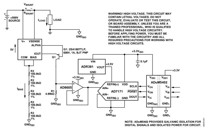
Figure 1. High Common-Mode Voltage Current Monitor (All Connections and Decoupling Not Shown)
