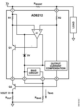
Figure 2. AD8212 High Voltage Operation Using an External PNP Transistor
