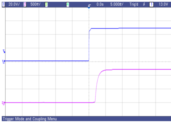
Fig. 57 AVO75-48S1V2 typical start-up from power on
