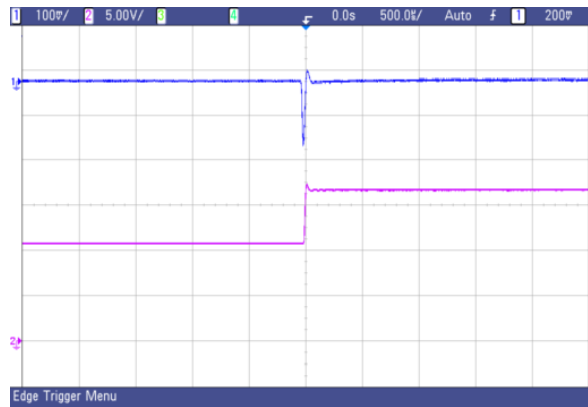
Fig. 45 AVO75-48S05 typical transient response to step increase in load from 50% to 75% of full load, room temperature, 48Vdc input ( \Delta I_o/\Delta t=1A/1\mu s )
