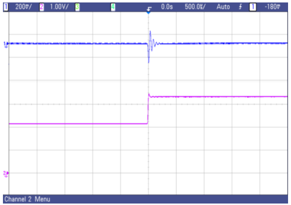
Fig. 25 AVO75-48S1V5 typical transient response to step increase in load from 50% to 75% of full load, room temperature, 48Vdc input ( \Delta I_o/\Delta t=1A/1\mu s )
