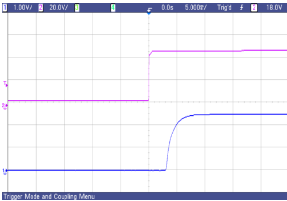
Fig. 63 AVO75-48S2V5 typical start-up from power on
