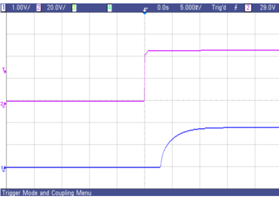
Fig. 61 AVO75-48S1V8 typical start-up from power on
