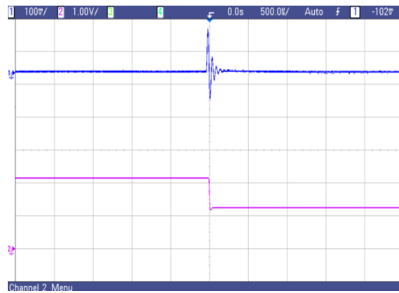
Fig. 24 AVO75-48S1V5 typical transient response to step decrease in load from 50% to 25% of full load, room temperature, 48Vdc input
