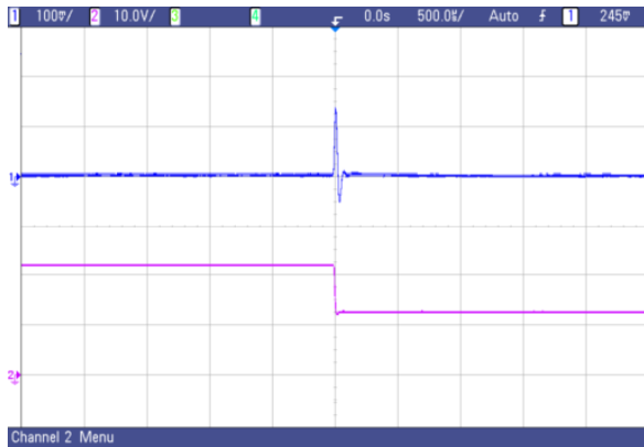
Fig. 36 AVO75-48S2V5 typical transient response to step decrease in load from 50% to 25% of full load, room temperature, 48Vdc input ( \Delta I_o/\Delta t=1A/1\mu s )
