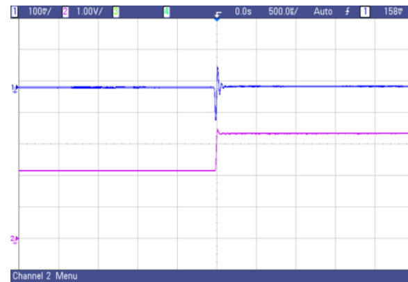
Fig. 33 AVO75-48S1V8 typical transient response to step increase in load from 50% to 75% of full load, room temperature, 48Vdc input ( \Delta I_o/\Delta t=1A/1\mu s )
