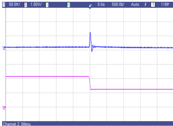
Fig. 22 AVO75-48S1V2 typical transient response to step decrease in load from 50% to 25% of full load, room temperature, 48Vdc input
