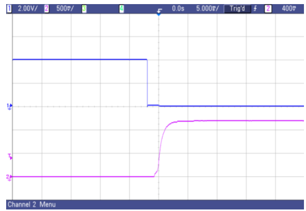
Fig. 58 AVO75-48S1V2 typical start-up from CNT on
