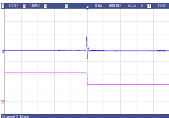
Fig. 32 AVO75-48S1V8 typical transient response to step decrease in load from 50% to 25% of full load, room temperature, 48Vdc input ( \Delta I_o/\Delta t=1A/1\mu s )
