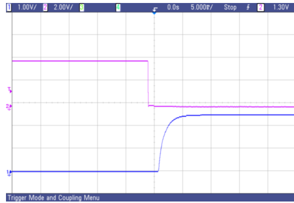
Fig. 64 AVO75-48S2V5 typical start-up from CNT on
