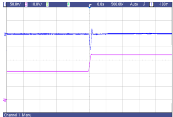
Fig. 35 AVO75-48S2V5 typical transient response to step increase in load from 50% to 75% of full load, room temperature, 48Vdc input ( \Delta I_o/\Delta t=0.1A/1\mu s )
