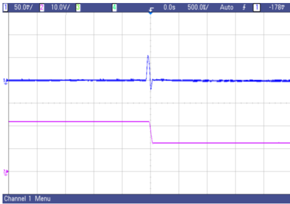
Fig. 34 AVO75-48S2V5 typical transient response to step decrease in load from 50% to 25% of full load, room temperature, 48Vdc input ( \Delta I_o/\Delta t=0.1A/1\mu s )
