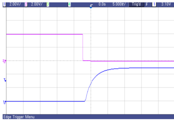
Fig. 68 AVO75-48S05 typical start-up from CNT on
