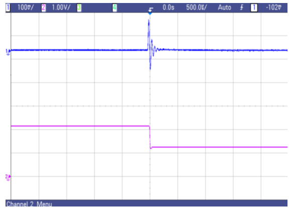
Fig. 24 AVO75-48S1V5 typical transient response to step decrease in load from 50% to 25% of full load, room temperature, 48Vdc input
