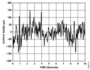
Figure 11.0.1 Hz to 10 Hz Output Noise, Shorted Inputs
