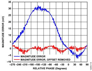
Figure 10. Magnitude Measurement Error vs. Relative Phase
