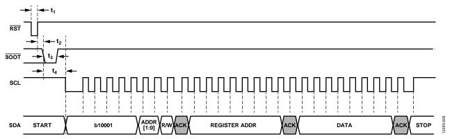
Figure 4. Load from EEPROM Timing Diagram
