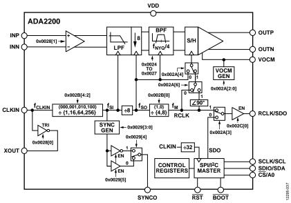
Figure 33. Detailed Block Diagram
