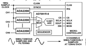
Figure 26. ADA2200 in an 8-Channel Simultaneous Sampling Application
