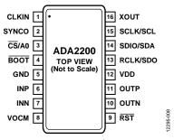
Figure 7. Pin Configuration
