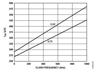
Figure 30. Typical Current Draw vs. CLKIN Frequency at  $V_{\rm DD}$  = 2.7 V and 3.3 V
