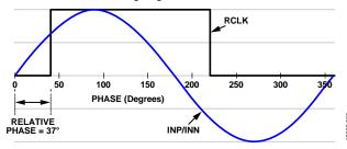
Figure 14. Example Showing Relative Phase,  $\theta_{REL}$ , of 37°
