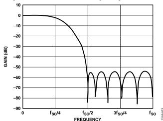
Figure 21. Decimation Filter Transfer Function, f<sub>SI</sub> = 800 kHz
