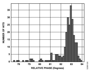
Figure 8. Histogram of Device-to-Device Phase Delay Variation
