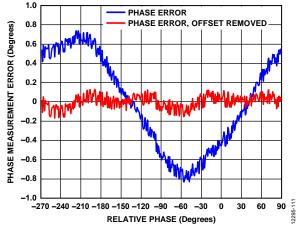
Figure 13. Phase Measurement Error vs. Relative Phase
