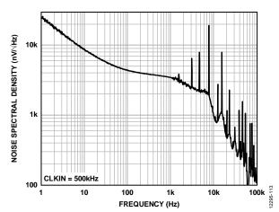
Figure 12. Noise Spectral Density vs. Frequency, fclkin = 500 kHz
