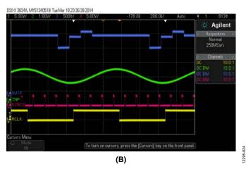
Figure 23. Output Sample Timing Relative to RCLK, (A) PHASE90 = 0, (B) PHASE90 = 1
