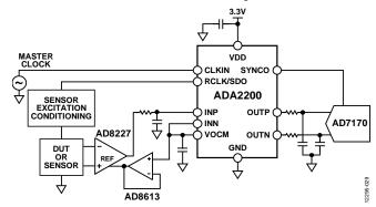
Figure 27. Lock-In Amplifier Application
