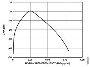
Figure 22. Default IIR Filter Frequency Response (fso/8 BPF)
