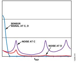
Figure 18. Output Spectrum of Synchronous Demodulator
