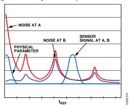
Figure 17. Output Spectrum of Synchronous Demodulator Before Demodulation
