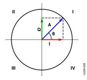
Figure 25. Rectangular and Polar Representation of a Signal
