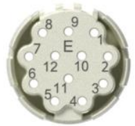
Contact Arrangement mating view
