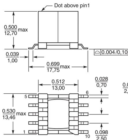
Dimensions are in  $\frac{\text{inches}}{\text{mm}}$
