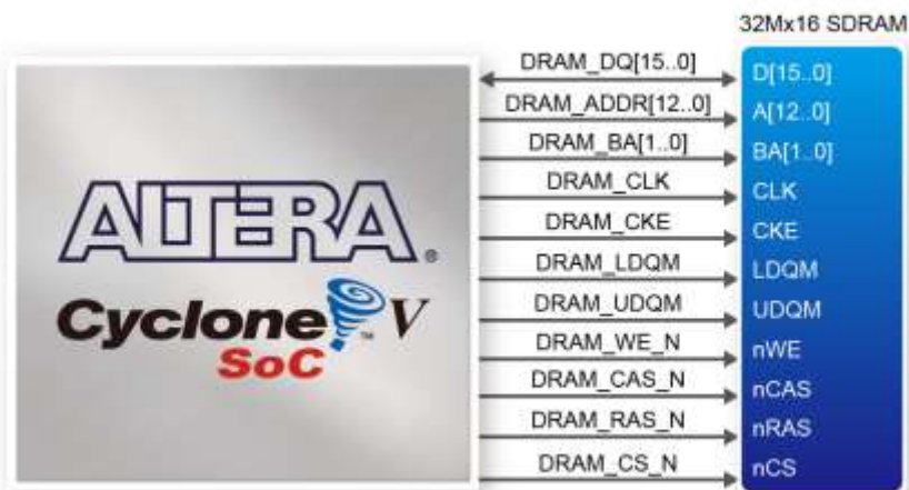
Figure 3-28 Connections between the FPGA and SDRAM
