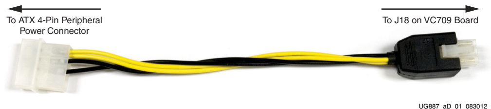
Figure D-1: ATX Power Supply Adapter Cable
