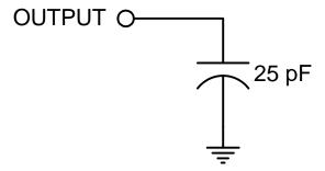
Figure 5.1 Output Equivalent Test Load
