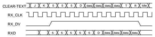
Figure 3.3 Relationship Between Received Data and Specific MII Signals
