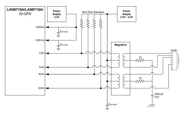
Figure 3.16 Twisted-Pair Interface Diagram (Dual Power Supplies)
