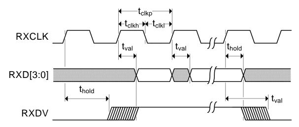
Figure 5.4 MII Receive Timing
