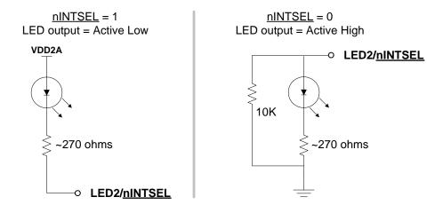
Figure 3.8 LED2/nINTSEL Polarity Configuration
