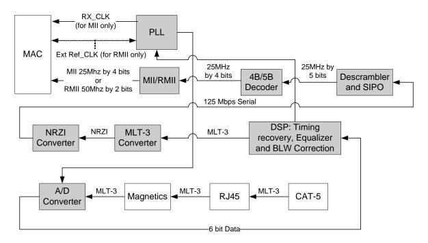
Figure 3.2 100BASE-TX Receive Data Path
