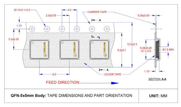
Figure 6.3 Taping Dimensions and Part Orientation
