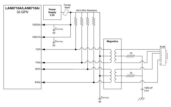
Figure 3.15 Twisted-Pair Interface Diagram (Single Power Supply)
