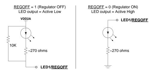
Figure 3.7 LED1/REGOFF Polarity Configuration
