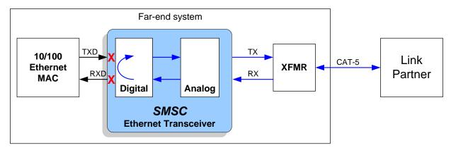
Figure 3.10 Far Loopback Block Diagram
