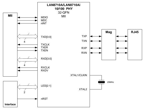
Figure 3.12 Simplified System Level Application Diagram
