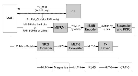
Figure 3.1 100BASE-TX Transmit Data Path
