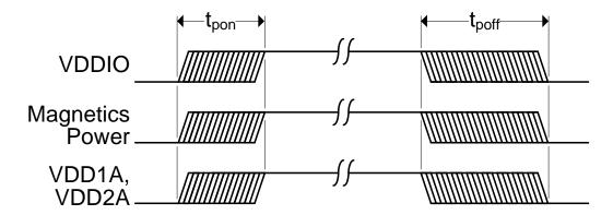
Figure 5.2 Power Sequence Timing
