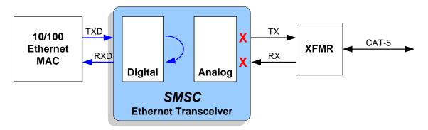
Figure 3.9 Near-end Loopback Block Diagram
