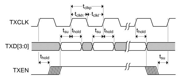
Figure 5.5 MII Transmit Timing
