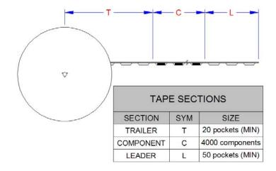
Figure 6.5 Tape Length and Part Quantity
