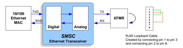
Figure 3.11 Connector Loopback Block Diagram
