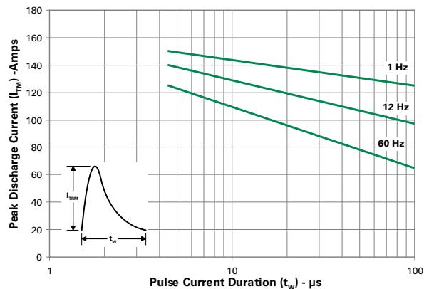
**Figure 11: Peak Repetitive Sinusoidal Pulse Current**
