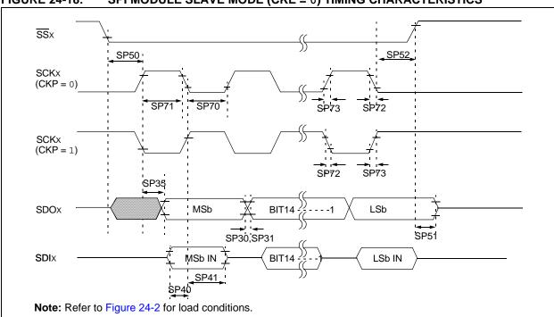
FIGURE 24-18: SPI MODULE SLAVE MODE (CKE = 0) TIMING CHARACTERISTICS
