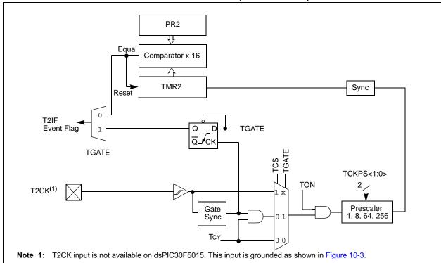
FIGURE 10-3: 16-BIT TIMER3 BLOCK DIAGRAM (TYPE C TIMER)
