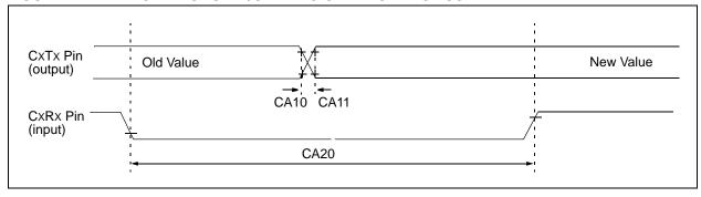
TABLE 24-39: CAN MODULE I/O TIMING REQUIREMENTS
