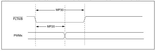
FIGURE 24-13: MOTOR CONTROL PWM MODULE TIMING CHARACTERISTICS
