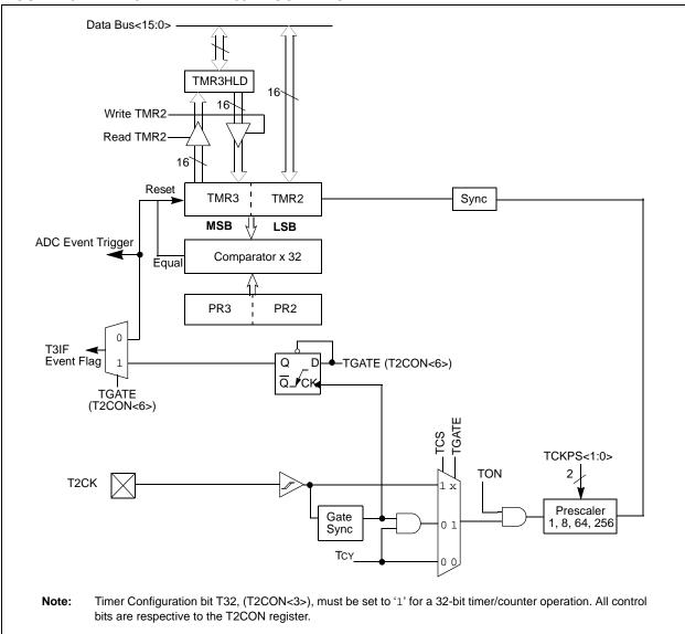
FIGURE 10-2: 16-BIT TIMER2 BLOCK DIAGRAM (TYPE B TIMER)
