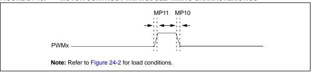
TABLE 24-30: MOTOR CONTROL PWM MODULE TIMING REQUIREMENTS
