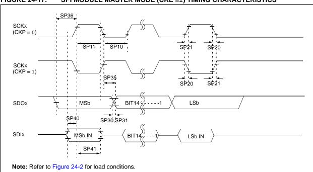
FIGURE 24-17: SPI MODULE MASTER MODE (CKE =1) TIMING CHARACTERISTICS
