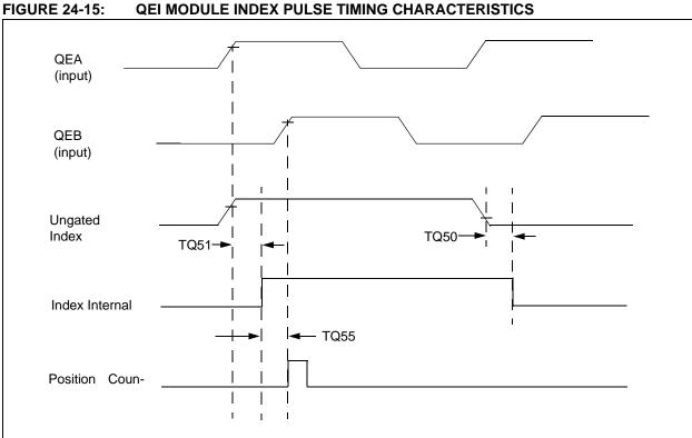
**QEI MODULE INDEX PULSE TIMING CHARACTERISTICS**
