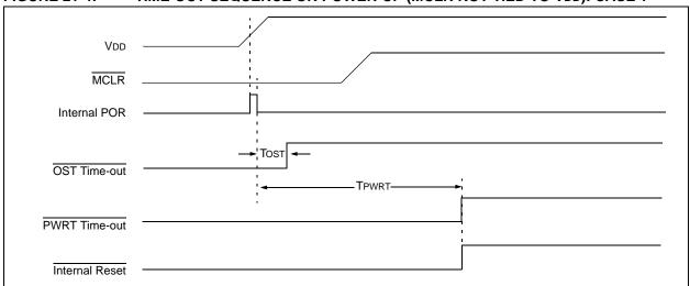
FIGURE 21-5: TIME-OUT SEQUENCE ON POWER-UP (MCLR NOT TIED TO VDD): CASE 2
