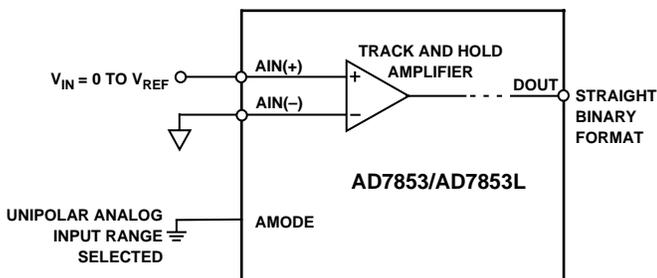
Figure 14. 0 to  $V_{REF}$  Unipolar Input Configuration
