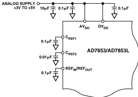
Figure 18. Relevant Connections When Using Internal Reference
