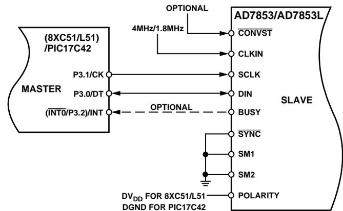
Figure 45. 8XC51/PIC17C42 Interface
