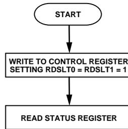
Figure 6. Flowchart for Reading the Status Register
