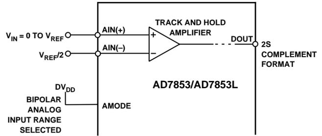
Figure 15.  $\pm V_{REF}/2$  about  $V_{REF}/2$  Bipolar Input Configuration
