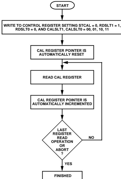
Figure 9. Flowchart for Reading from the Calibration Registers
