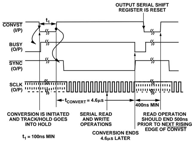
Figure 38. Mode 4, 5 Timing Diagram ( $SM1 = 1, SM2 = 1$  and 0)
