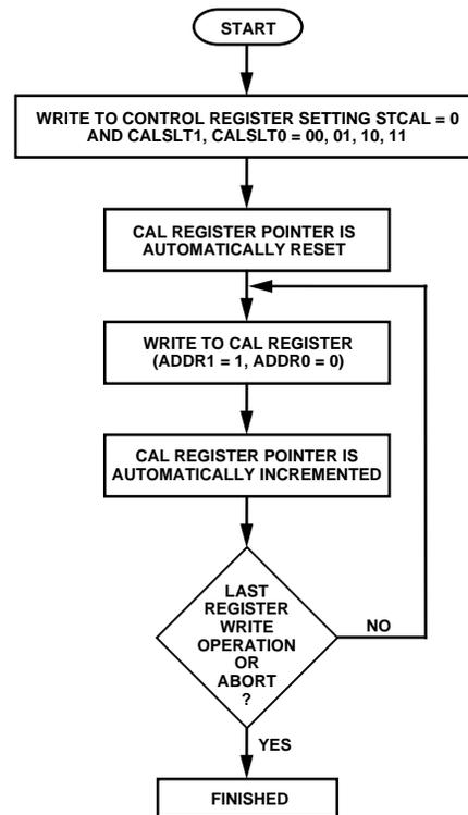
*Figure 8. Flowchart for Writing to the Calibration Registers*
