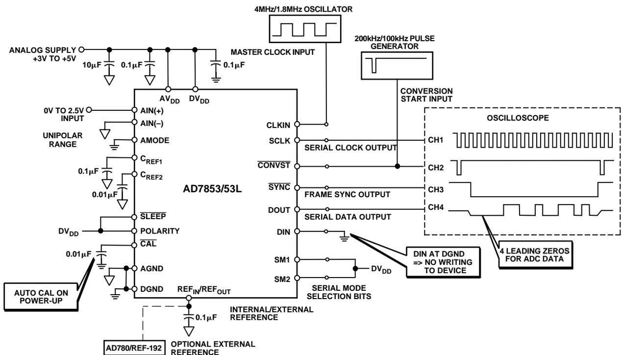
Figure 10. Typical Circuit
