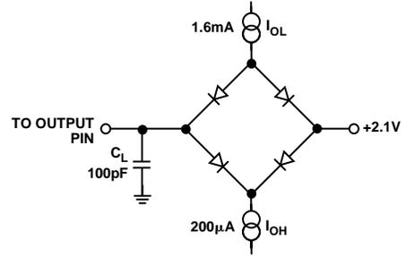
Figure 1. Load Circuit for Digital Output Timing Specifications
