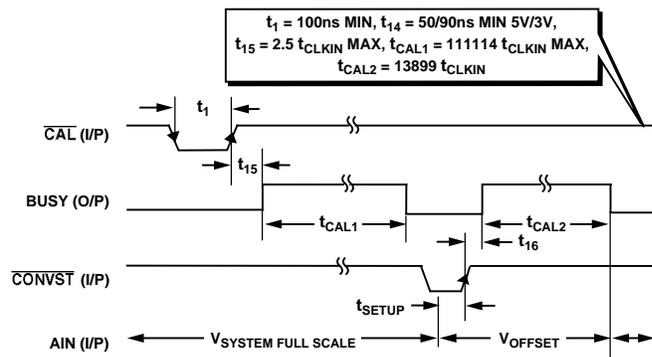
Figure 31. Timing Diagram for Full System Calibration
