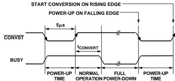
Figure 24. Power-Up Timing When Using  $\overline{CONVST}$  Pin
