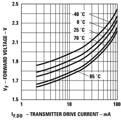
Figure 2. Typical Forward Voltage vs Drive Current
