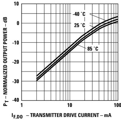
Figure 3. Typical Normalized Optical Power vs Drive Current
