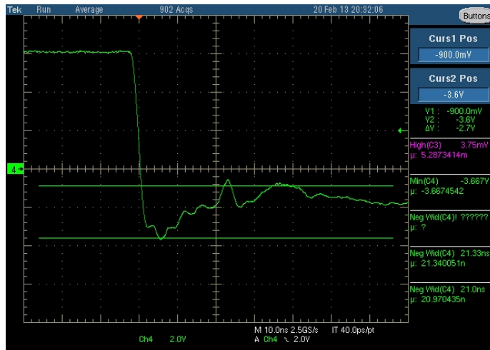
Figure 4. Typical Reverse Recovery I_F = 1.5 \text{ A} to V_R = 28 \text{ V}
