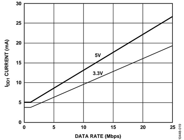
Figure 19. Typical ADuM7643 V<sub>DD1</sub> or V<sub>DD2</sub> Supply Current vs. Data Rate for 5 V and 3.3 V Operation
