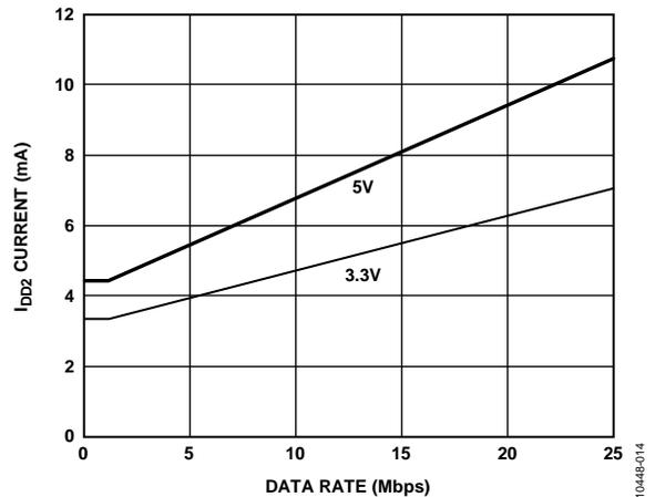
Figure 14. Typical ADuM7640 V<sub>DD2</sub> Supply Current vs. Data Rate for 5 V and 3.3 V Operation
