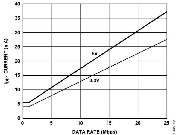
Figure 15. Typical ADuM7641 V<sub>DD1</sub> Supply Current vs. Data Rate for 5 V and 3.3 V Operation
