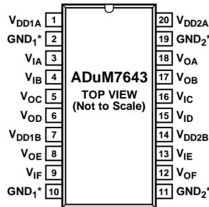
\*PIN 2 AND PIN 10 ARE INTERNALLY CONNECTED. CONNECTING BOTH PINS TO PCB SIDE 1 GROUND IS RECOMMENDED. PIN 11 AND PIN 19 ARE INTERNALLY CONNECTED. CONNECTING BOTH PINS TO PCB SIDE 2 GROUND IS RECOMMENDED.
