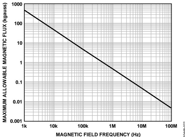
Figure 22. Maximum Allowable External Magnetic Flux Density
