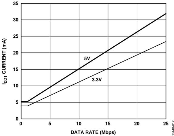
Figure 17. Typical ADuM7642 V<sub>DD1</sub> Supply Current vs. Data Rate for 5 V and 3.3 V Operation
