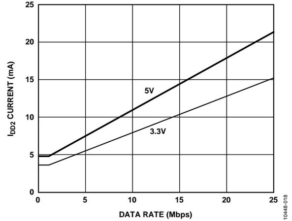
Figure 18. Typical ADuM7642 V<sub>DD2</sub> Supply Current vs. Data Rate for 5 V and 3.3 V Operation
