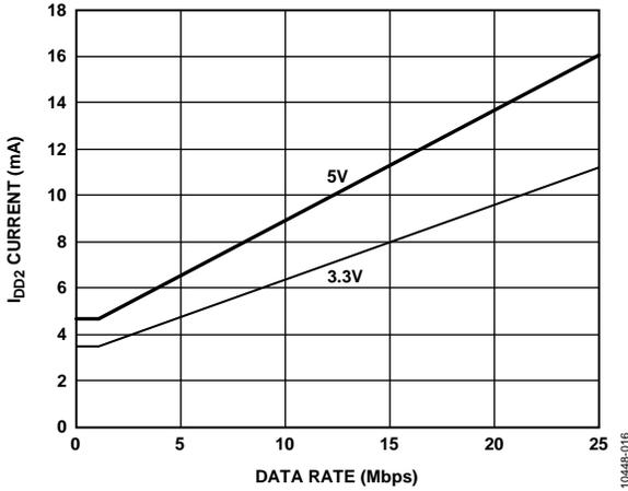
Figure 16. Typical ADuM7641 V<sub>DD2</sub> Supply Current vs. Data Rate for 5 V and 3.3 V Operation
