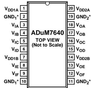
\* PIN 2 AND PIN 10 ARE INTERNALLY CONNECTED. CONNECTING BOTH PINS TO PCB SIDE 1 GROUND IS RECOMMENDED. PIN 11 AND PIN 19 ARE INTERNALLY CONNECTED. CONNECTING BOTH PINS TO PCB SIDE 2 GROUND IS RECOMMENDED.
