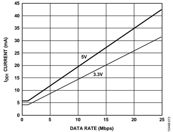
Figure 13. Typical ADuM7640 V<sub>DD1</sub> Supply Current vs. Data Rate for 5 V and 3.3 V Operation
