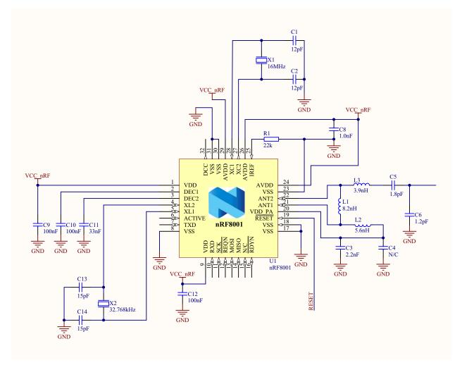
Figure 22. nRF8001 schematic, without DC/DC converter enabled
