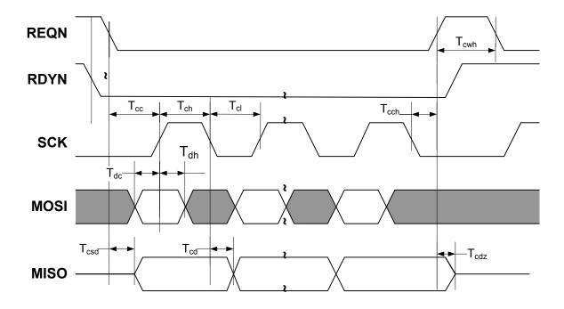
Figure 13. nRF8001 initiated packet SPI timing
