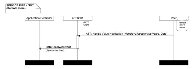
Figure 38. Data transfer on a receive pipe; data stored remotely
