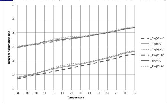
Figure 15. shows the current consumption in RX and TX mode over the full temperature sensor range.
