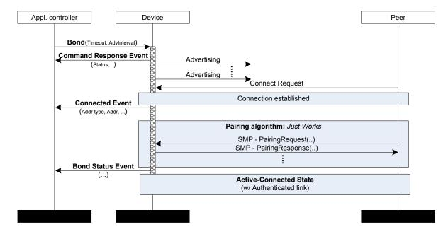
Figure 48. Bonding procedure MSC
