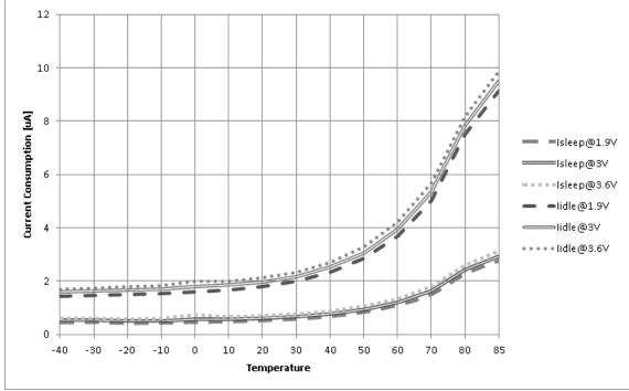
Figure 16. Current consumption in lidle and Isleep with DC/DC converter not active
