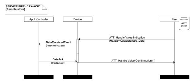
Figure 39. Data transfer on a receive pipe; acknowledgment enabled and data stored remotely
