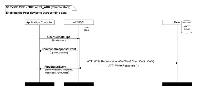
Figure 33. Receive pipe opening; data stored remotely
