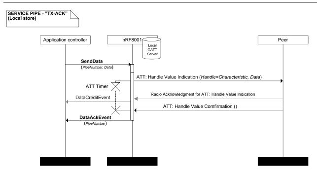
Figure 29. Data transfer on a transmit pipe; acknowledgment enabled and data stored locally
