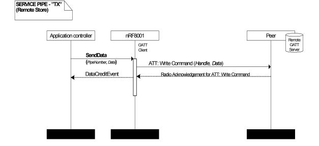
Figure 30. Data transfer on a transmit pipe; data stored remotely
