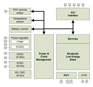
Figure 1. nRF8001 block diagram
