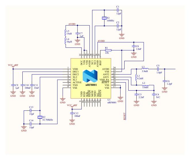
Figure 21. nRF8001 schematic, with DC/DC converter enabled
