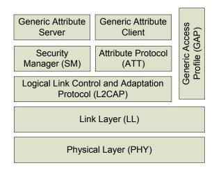
Figure 2. Bluetooth low energy layers implemented in nRF8001
