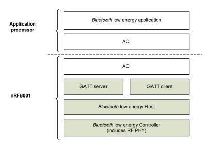
Figure 23. nRF8001 ACI connectivity
