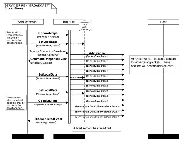
Figure 32. Broadcasting data on a service pipe; data stored locally
