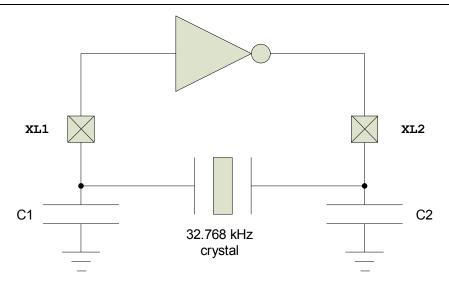
Figure 5. Circuit diagram of the nRF8001 32.768 kHz crystal oscillator
