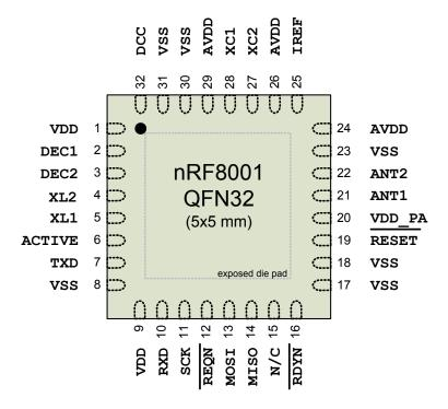
Figure 3. nRF8001 pin assignment (top view)
