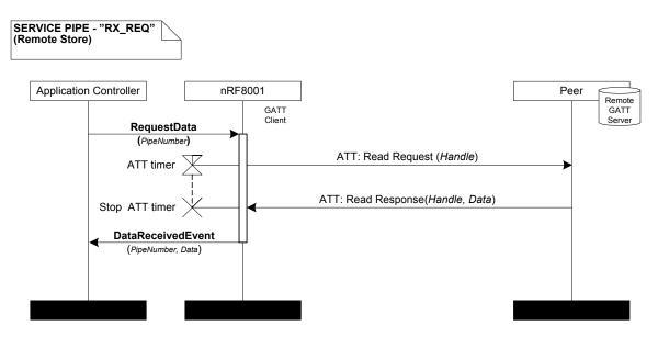
Figure 41. Data transfer on a receive pipe after data request received, data stored remotely
