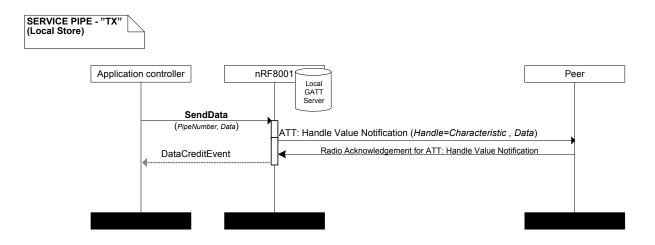
Figure 28. Data transfer on a transmit pipe; data stored locally
