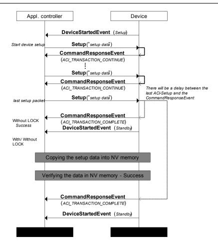
Figure 44. Setup procedure MSC
