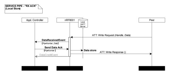
Figure 36. Data transfer on a receive pipe; acknowledgment enabled and data stored locally
