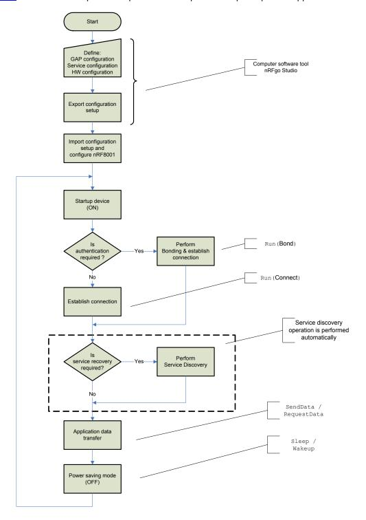
Figure 50. Normal configuration and connection establishment procedure (example)
