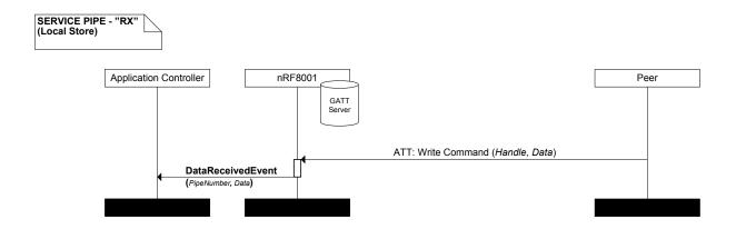
Figure 35. Data transfer on a receive pipe; data stored locally
