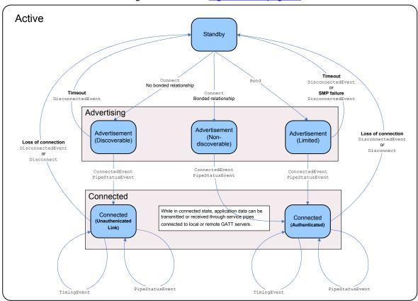
Figure 47. Active mode operation state machine
