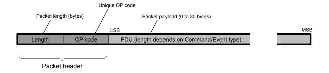
Figure 25. ACI packet structure
