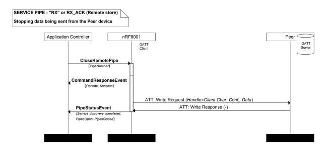
Figure 34. Receive pipe closing; data stored remotely
