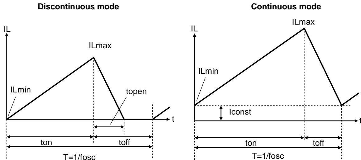
There are two operation modes of the step-up PWM control-DC/DC converter. That is the continuous mode and discontinuous mode by the continuousness inductor.
