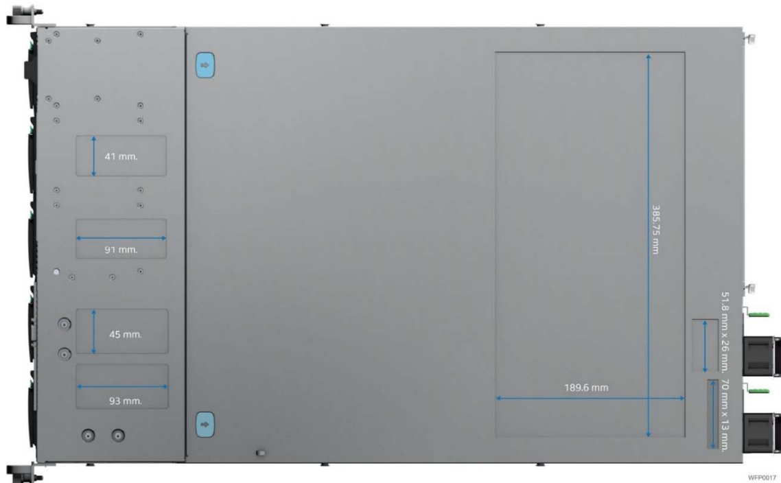
Figure 14. Label Emboss Dimensions
