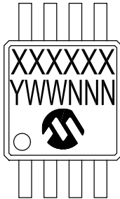
8-Lead SOIC (150 mil) (MCP661, MCP662, MCP663)
