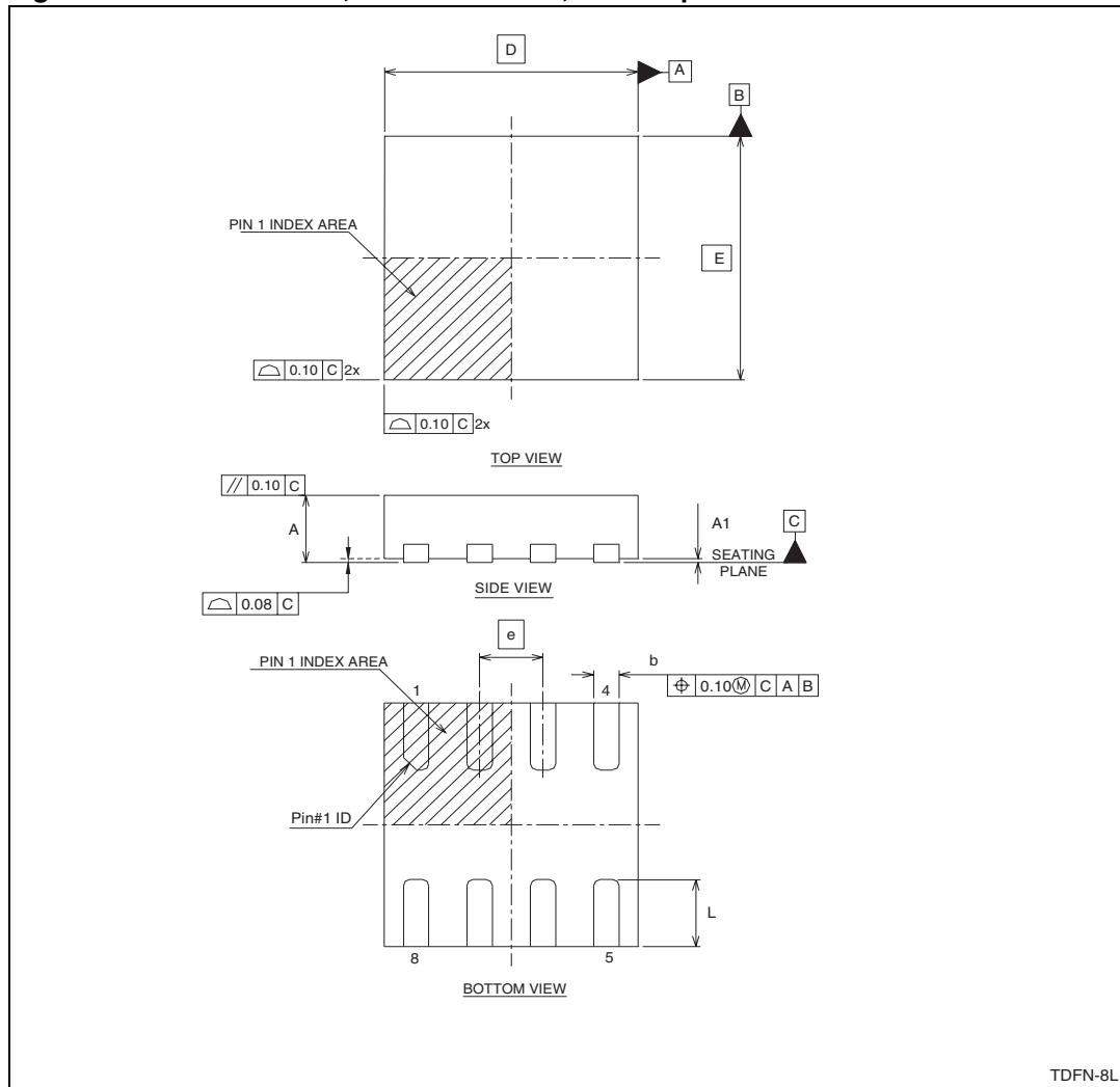
**Table 7. TDFN – 8-lead 2 x 2 x 0.75 mm, 0.5 mm package mechanical data**
