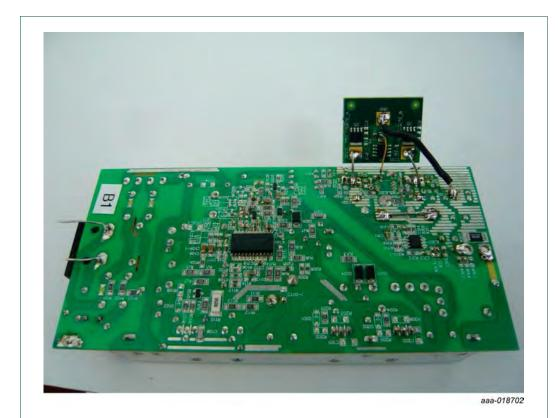
Fig 6. TEA1995DB1295 demo board connected to 150 W resonant adapter board APBADC069
