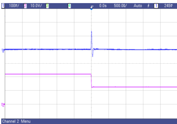
Fig.36 AVO505-48S2V5 typical transient response to step decrease in load from 50% to 25% of full load, room temperature, 48Vdc input ( \Delta I_o/\Delta t = 1A/1\mu s )
