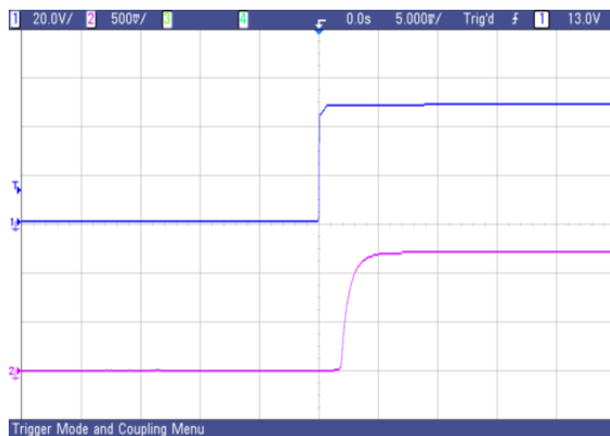
Fig.57 AVO50-48S1V2 typical start-up from power on
