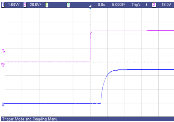
Fig.63 AVO50-48S2V5 typical start-up from power on
