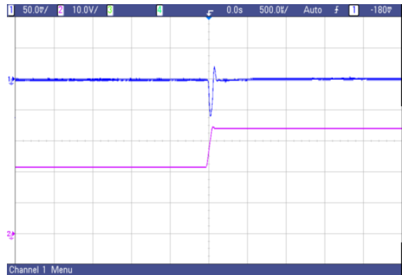
Fig. 35 AVO50-48S2V5 typical transient response to step increase in load from 50% to 75% of full load, room temperature, 48Vdc input ( \Delta I_o/\Delta t = 0.1A/1\mu s )
