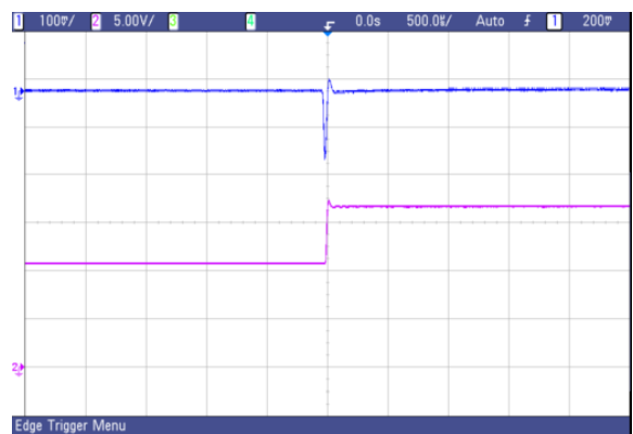
Fig.45 AVO50-48S05 typical transient response to step increase in load from 50% to 75% of full load, room temperature, 48Vdc input ( \Delta I_o/\Delta t = 1A/1\mu s )
