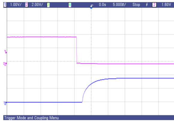
Fig.62 AVO50-48S1V8 typical start-up from CNT on
