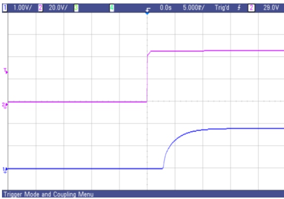
Fig.61 AVO50-48S1V8 typical start-up from power on
