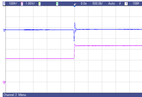
Fig.33 AVO50-48S1V8 typical transient response to step increase in load from 50% to 75% of full load, room temperature, 48Vdc input ( \Delta I_o/\Delta t = 1A/1\mu s )
