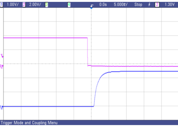
Fig.64 AVO50-48S2V5 typical start-up from CNT on
