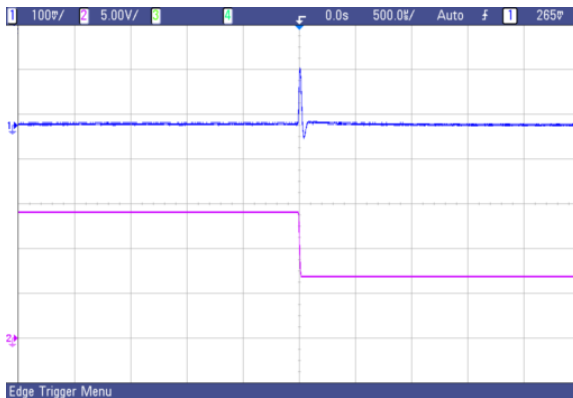
Fig.44 AVO50-48S05 typical transient response to step decrease in load from 50% to 25% of full load, room temperature, 48Vdc input ( \Delta I_o/\Delta t = 1A/1\mu s )
