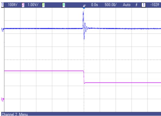
Fig.24 AVO50-48S1V5 typical transient response to step decrease in load from 50% to 25% of full load, room temperature, 48Vdc input ( \Delta I_o/\Delta t = 1A/1\mu s )
