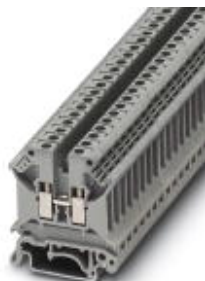
Feed-through terminal block, Connection method: Screw connection, Cross section: 0.2 mm 2 - 6 mm 2 , AWG: 24 - 10, Width: 6.2 mm, Color: black/yellow, Mounting type: NS 35/7,5, NS 35/15, NS 32
