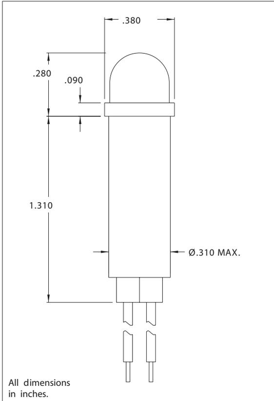
Solid-state indicator lights complete with built-in current-limiting resistor and rectifier diode.
